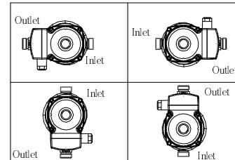
Keep the Pump Shaft Parallel to Sea Level
